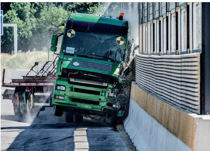
DB NBF system in a crash test: The top product in the portfolio of the Kirchdorf Road & Traffic division combines the tried-and-tested DELTABLOC® impact protection with noise protection elements, which can be integrated with flexible design and choice of materials.
