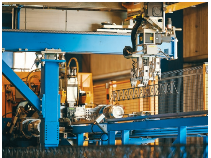
Modern technology, high added value: The mesh welding plant was replaced and the new lattice girder welding plant increases added value.
