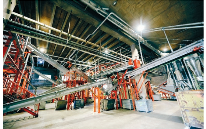
Managing Director Christian Zirgoi shows us how the tires, which are crisscrossed with steel wires, are gradually disassembled into their component parts.
