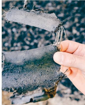
Managing Director Christian Zirgoi shows us how the tires, which are crisscrossed with steel wires, are gradually disassembled into their component parts.
