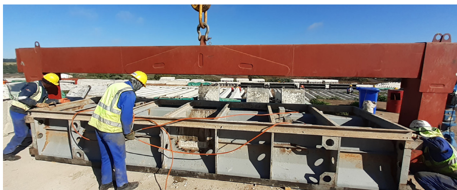
The mobile turning unit is a core component of the unique South African TPP system.
