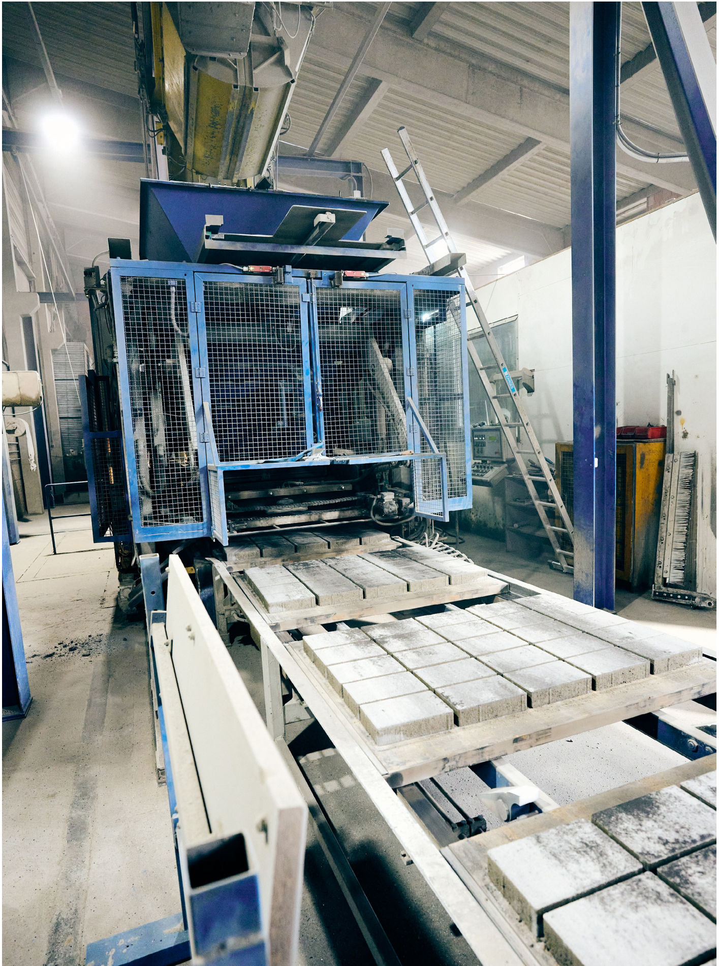
Automated and specialized: the impressive Zenith paving machine has for years been the workhorse for one of the most successful product groups of the traditional precast manufacturer in Leoben. Further investments will soon be made to integrate the site even better into the Kirchdorfer Concrete Solutions product range with new product developments.
